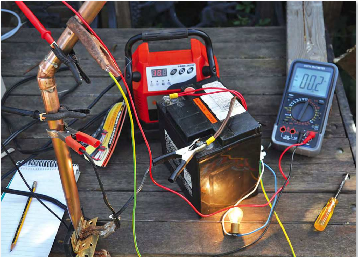
Fig 2: Method of testing a copper pipe joint using 10A battery charger. The bulb provides a current limiting load to prevent the battery over-charging during the test.
